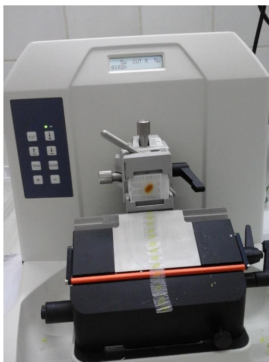
Figure 60: Microtome SLEE CUT 6062 (photo originale)
