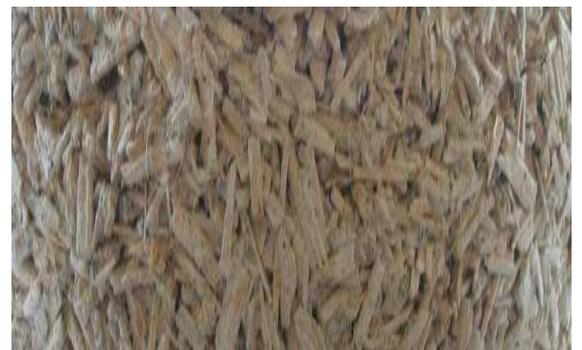
**Figure I.10 béton chanvre**
