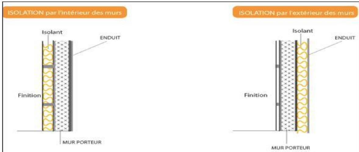
**Figure I.7: Isolation intérieure et extérieure des murs / source** [https://www.google.com/search?hl=fr-](https://www.google.com/search?hl=fr-DZ&biw=1366&bih=608&tbm=isch&sa=1&ei=h3LMXPrKPiTlwTPgJTYCg&q=L%E2%80%99isolation+par+l%E2%80%99ext%C3%A9rieur+%&coq=L%E2%80%99isolation+par+l%E2%80%99ext%C3%A9rieur+%gs_l=img.3...51524.51524..55045...0.0.0.87.87.1.....1...2j1.gws-wiz-)
