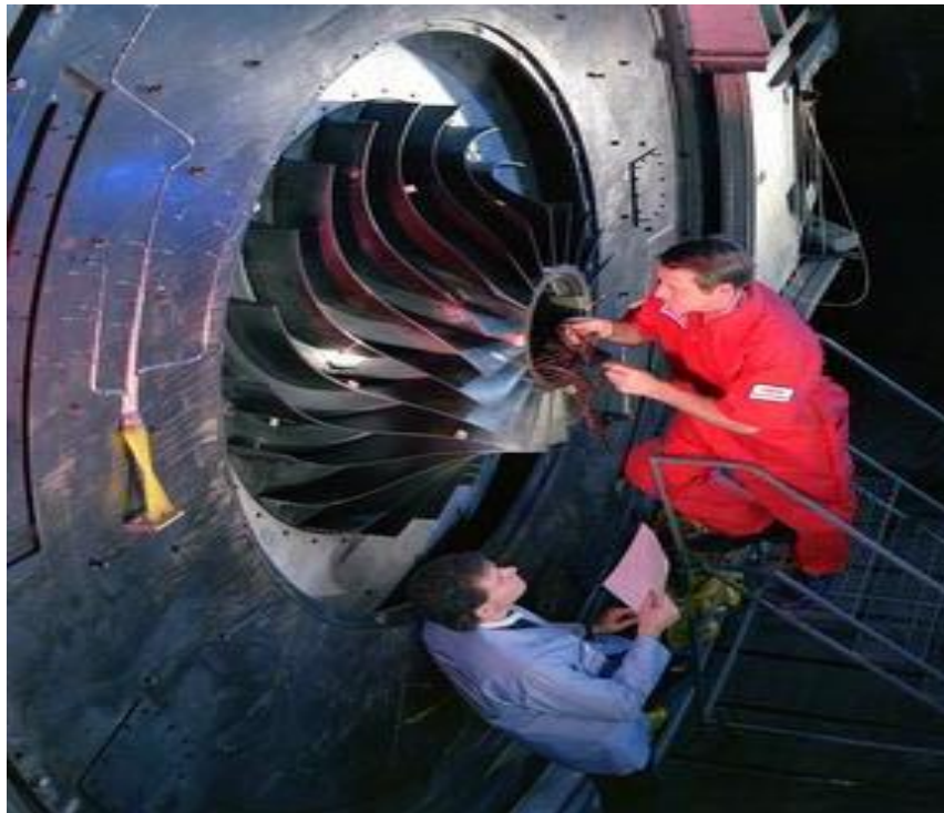
Figure 1.4 : compresseur centrifuge (Low-Speed Centrifugal Compressor (LSCC) in NASA) [12]
