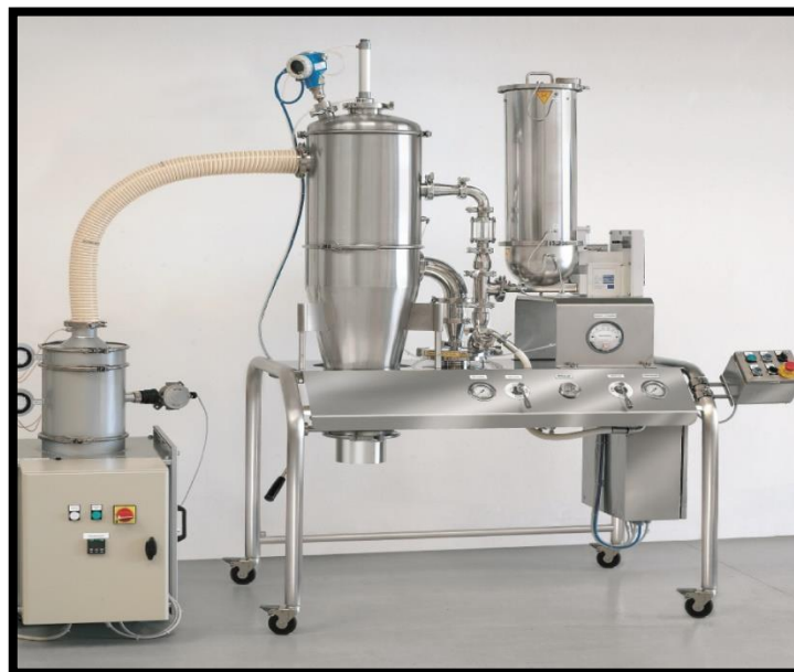
Figure 2.7 Micronization Mill/ Spiral Jet Mill[54]
