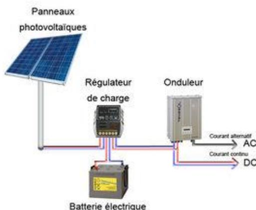
Figure I-19 : Installation photovoltaïque autonome. [8]
