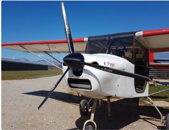
Figure I-9 : Les hélices carbone-titane E-PROPS.
