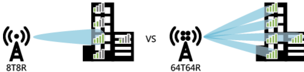
Figure 3- 3: Massive MIMO 8T8R&64T64R [14].
