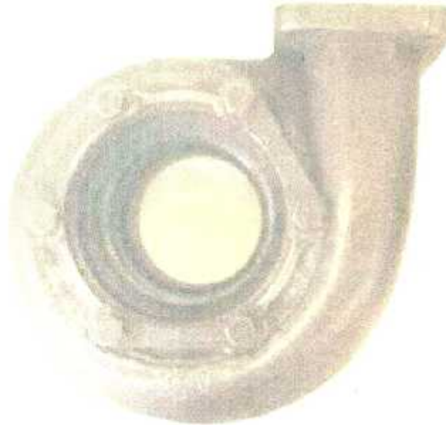
Figure 4-10 :Le logement turbine
