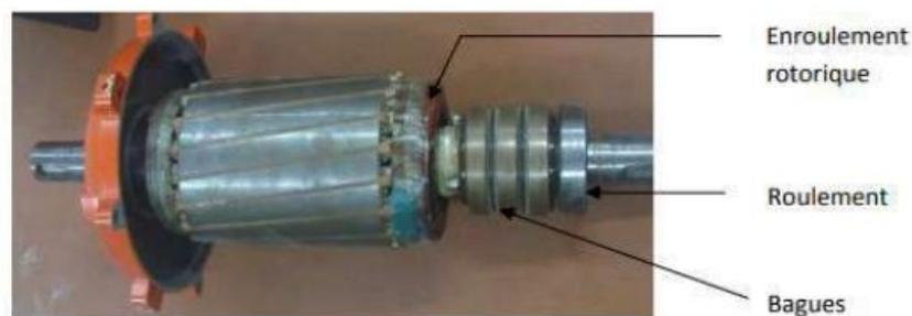
**Fig (1.8) :** rotor bobiné
