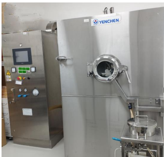
Figure III.9 : Turbine de pelliculage
