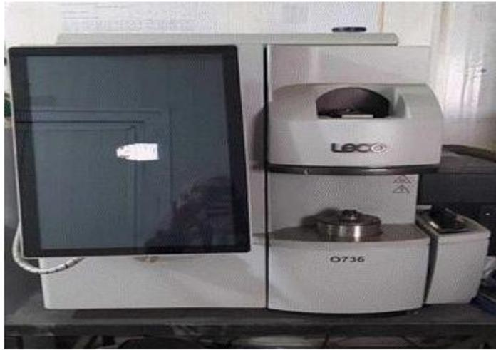
**Figure 3.2 :** Appareil Oxygen/Nitrogen System.
