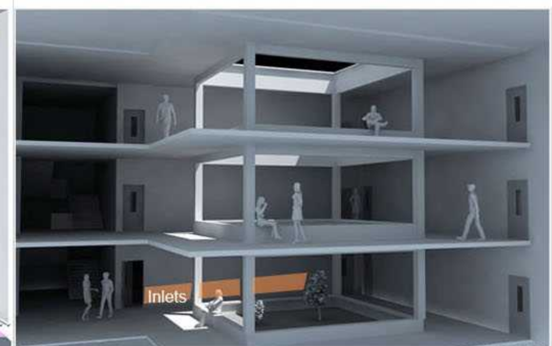
Location of inlets on the interior southern wall Classroom 101 A ;Ventilation inlet at courtyard base
