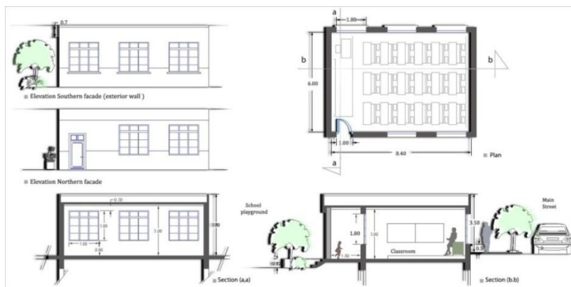
Fig.111. Elevation Plans and cross-section of a typical classroom showing the location, dimension, types and form of fenestration openings.
