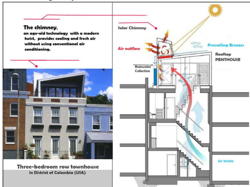
Fig 88. Ex of Solar Chimney incorporated on a staircase (Source: Google image adapted by author)
