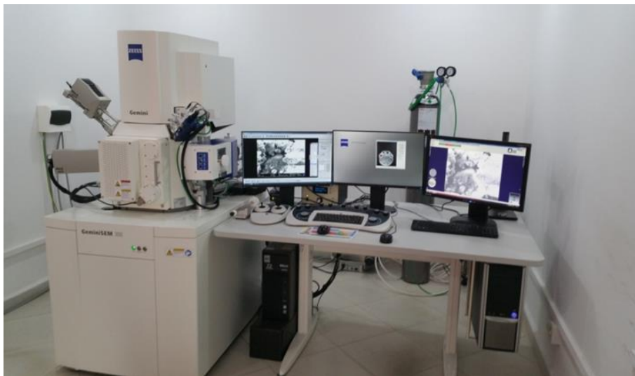
Figure 2.5: Equipment of the SEM apparatus equipped with an EDS analyzer.(CRTI)
