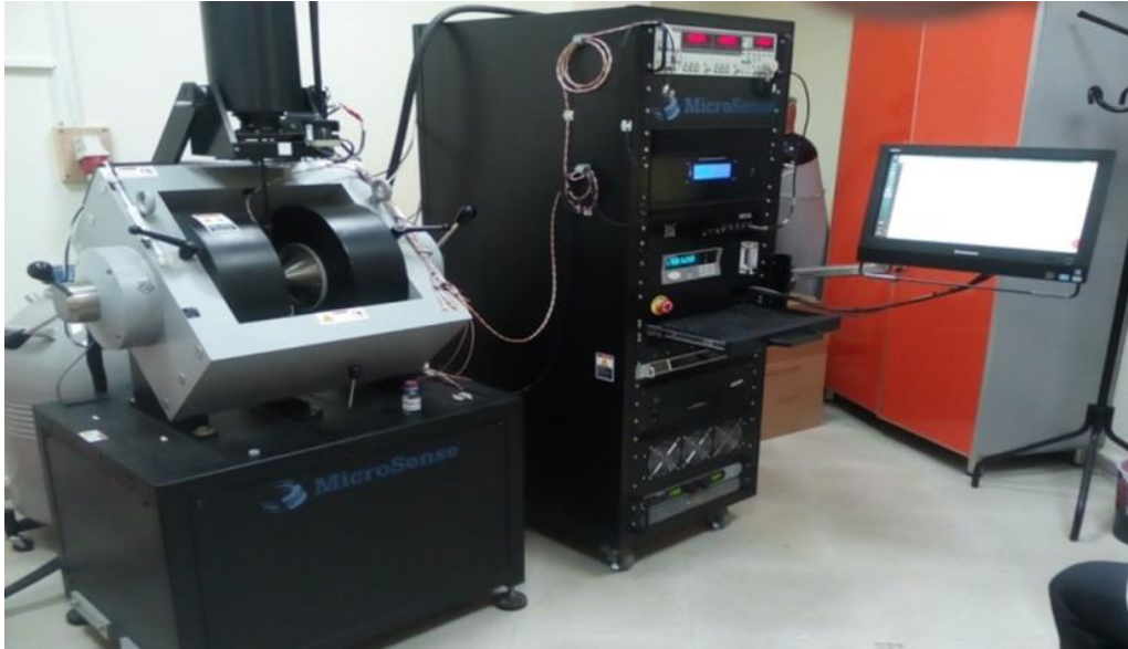
Figure 2.12: Vibrating sample magnetometer (VSM).(CRTI)
