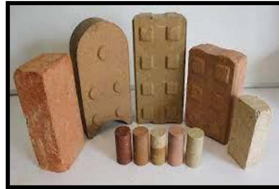
Figure143 : brique BTC Source : https://www.futura-sciences.com/maison/definitions/construction-maison-brique-btc-17851/
