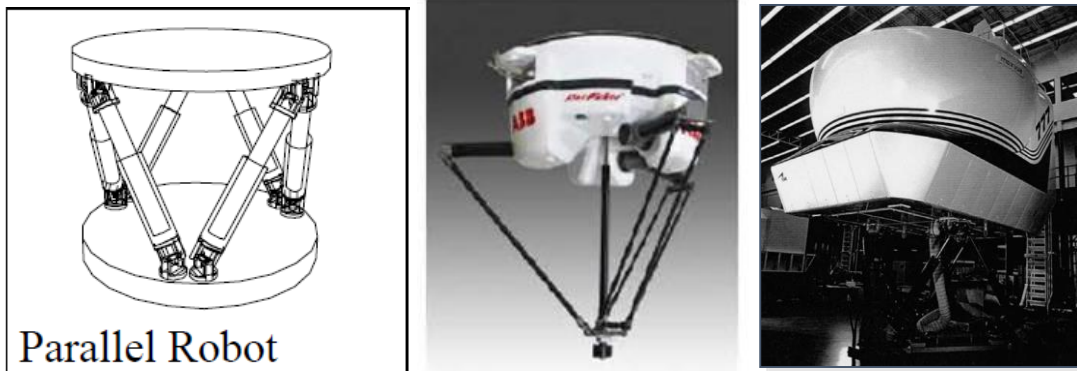
Figure 1-6 Examples of parallel robots
