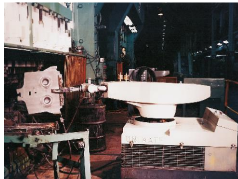
Figure 1- 1 Universal automation, the first Unimation robot working at a General Motors factory [1]
