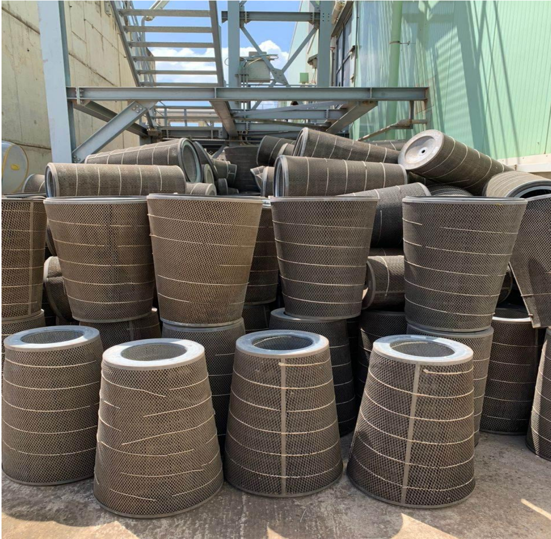
Figure 2.10: Cartouches colmaté (originale 2023)
