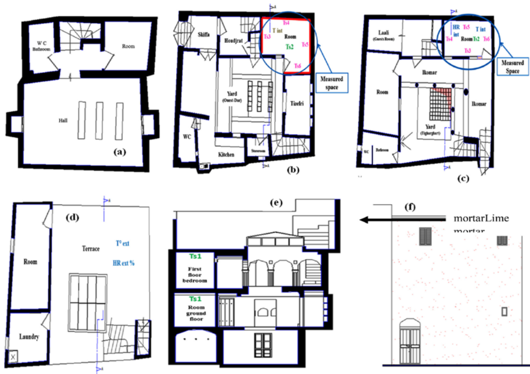
Figure II.6: House plan: (a) Basement plan, (b) Ground floor plan, (c) First floor plan, (d) Terrace plan, (e) Section AA, (f) Façade.
