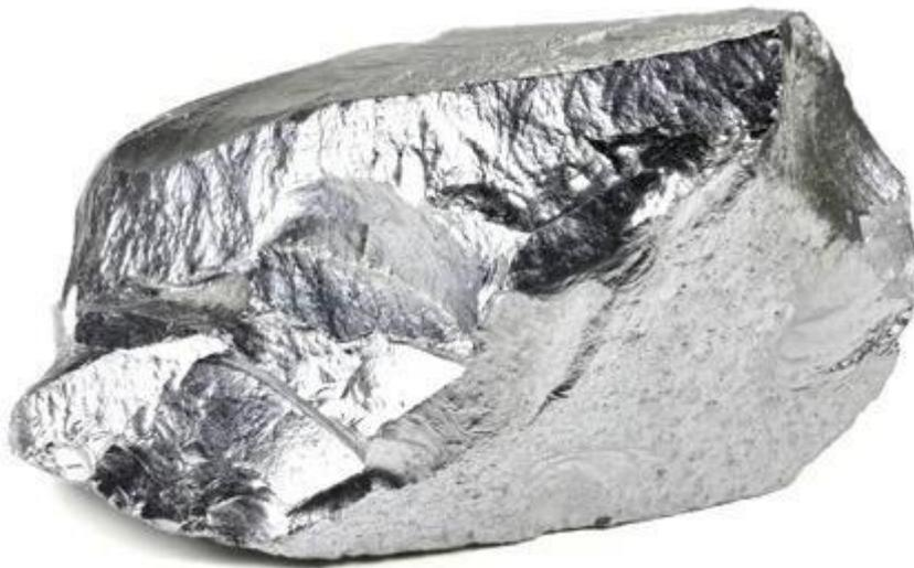
**Figure (I.26) :** le silicium poly cristallin
