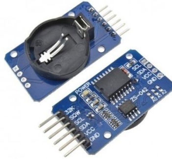
Figure III.19: RTC (Real Time Clock).[62]
