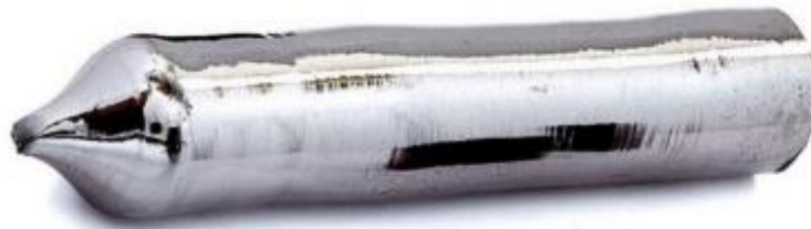
Figure I-15: Lingot cylindrique de silicium monocristallin [53]
