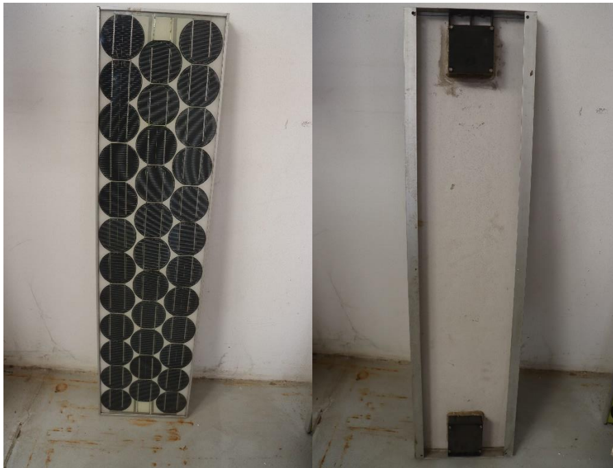
Figure III -1: Panneau ARCO de 35 Cellules rondes (CRTSE)
