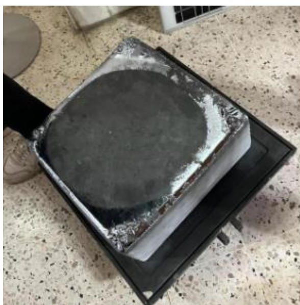
Figure I-16: Lingot de silicium multicristallin 40 cm × 40 cm × 18 cm (CRTSE)
