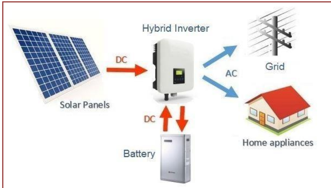
Figure 1.12 : Hybrid solar system [25].
