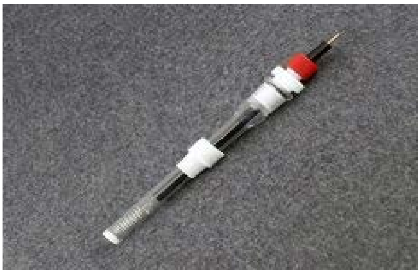
Figure 1.5: Photograph of counter electrode. [18]
