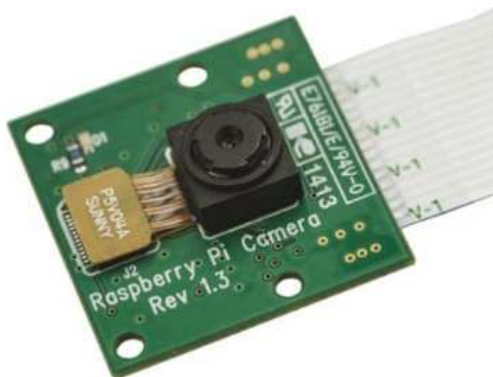
Figure 2.24 Le module camera Raspberry Pi V1.3.
