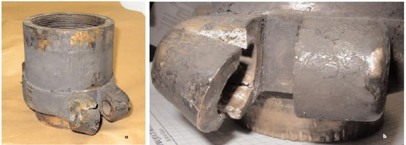
Figure 1.3: (a) Ductile Fracture of 2 1/2 Inch Hose Fitting (b) Close-up of the Deformed Region Where a Pin Joining the “Ears” Became Free from the One on the Right Causing the Deformation and Fracture of the One on the Left (Photos Courtesy of Sachs, Salvaterra & Associates, Inc.)
