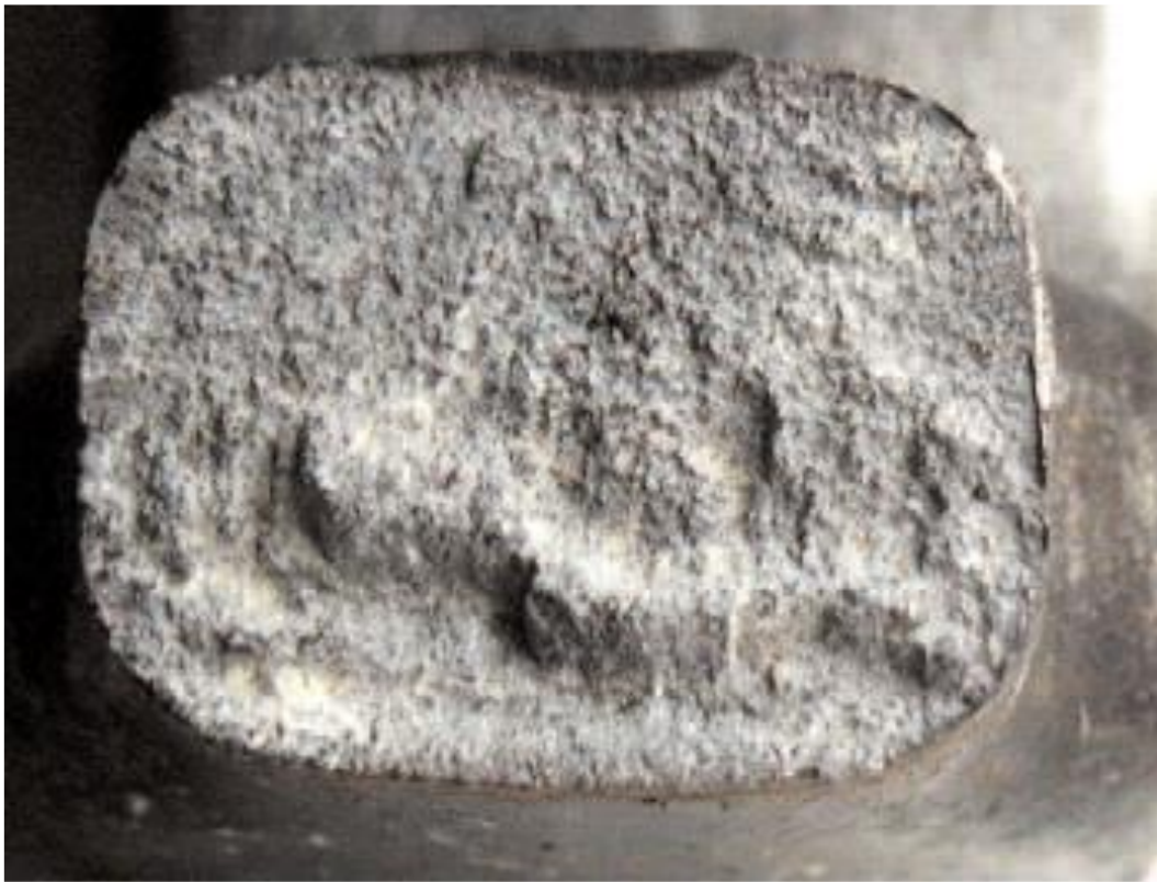
Figure 1.2: Brittle Fracture Surface of a High-Strength Chain. Fracture Began in a Small Crack Resulting from a Heat-Treating Problem (Photo Courtesy of Sachs, Salvaterra & Associates, Inc.).
