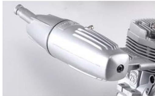
A newly designed "POWER BOX" silencer is supplied with the engine that offers not only quieter and milder exhaust sound but excellent power as well. Also, the exhaust outlet direction can be rotated to meet specific applications.
