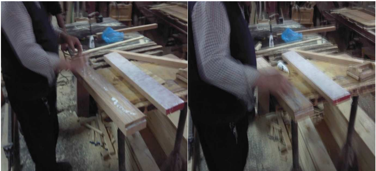
Figure IV-A-4 : Collage des planches
