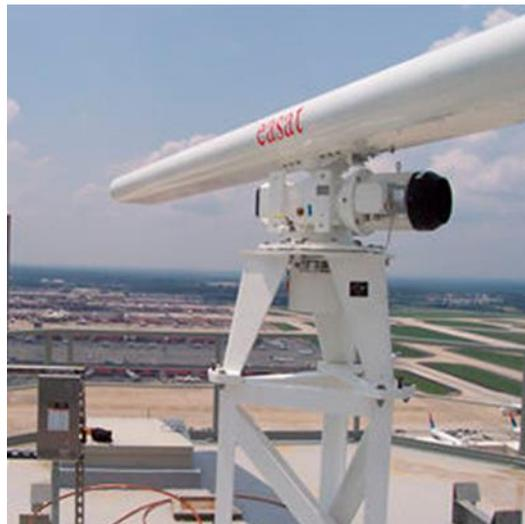
**Figure I.8 :** Radar de surface
