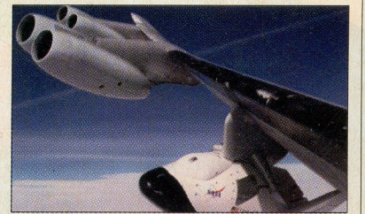
NASA ISS "lifeboat" X-38 is carried by B-52
