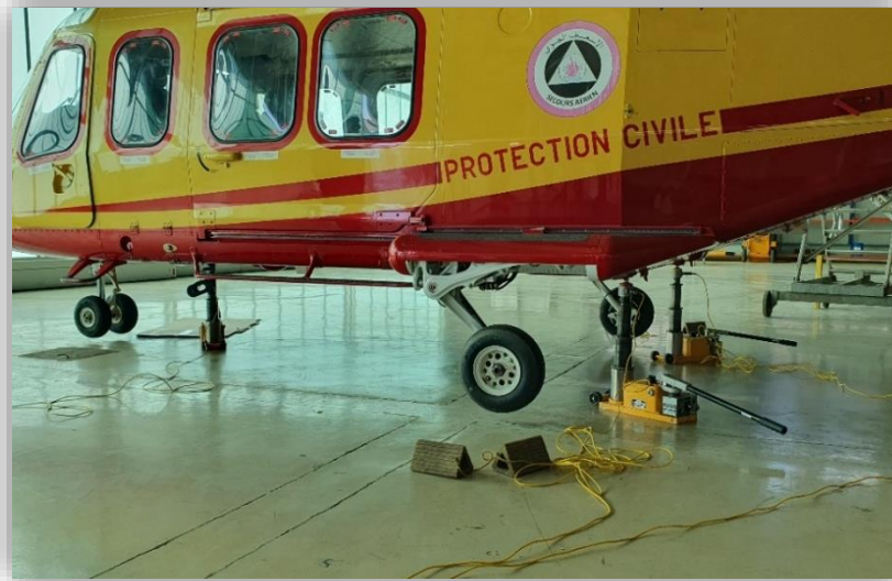
Figure 4.23: Helicopter lifted by three jacks related to scales
