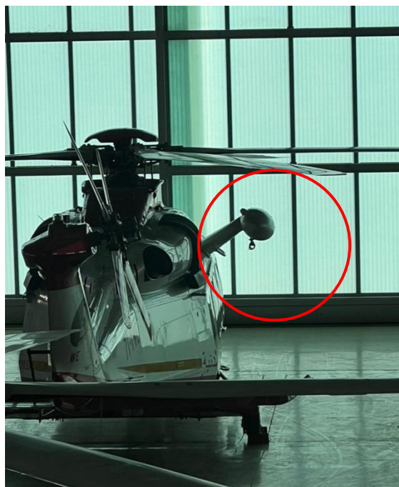
Figure E.4: Hoist Breeze implemented on AW139
