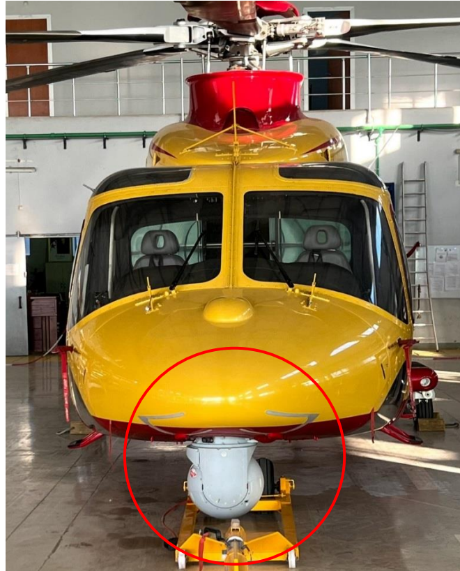
Figure E.8: Flir wes camera implemented on AW139
