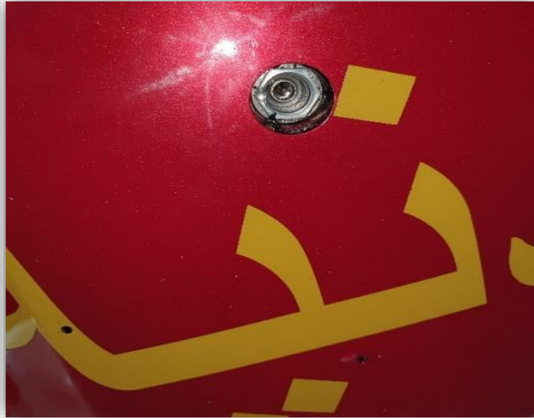
Figure 4.8: Defueling evacuation hole
