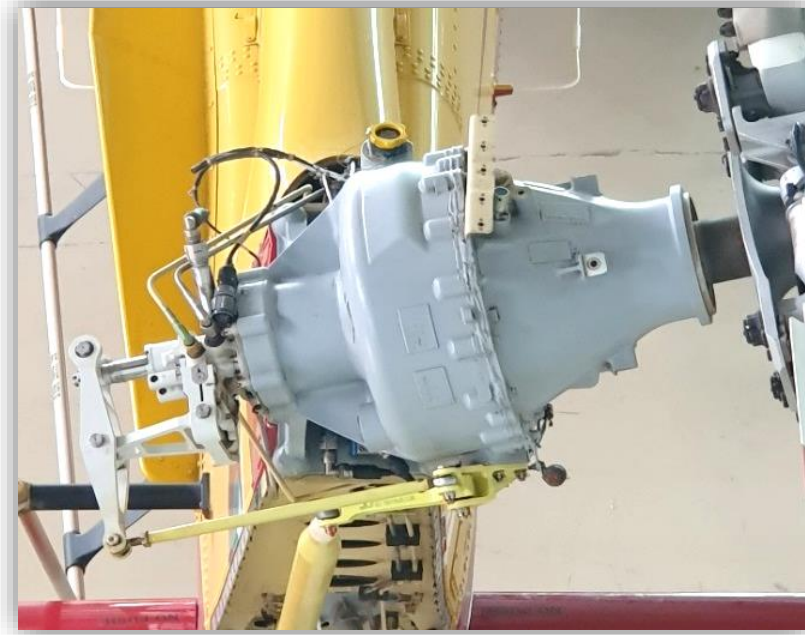
Figure 4.12: The tail gearbox's oil gauge
