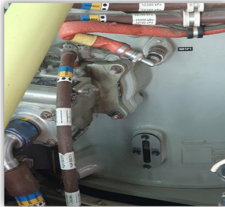
Figure 4.10: The main gearbox's oil gauge
