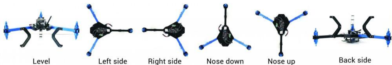
Figure 2.17 Accelerometer and Compass calibration positions for copter [83].
