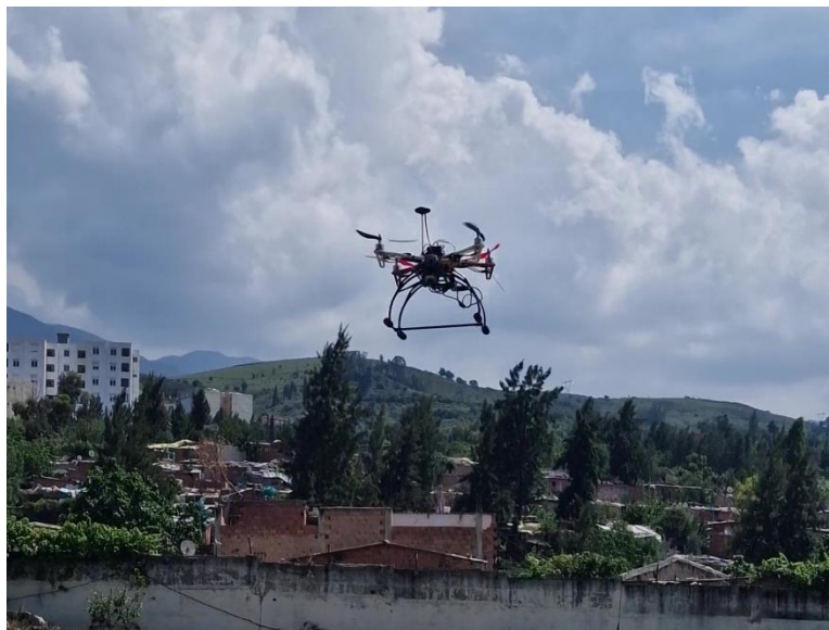
Figure 4.4 Our quadcopter surveying the AOI 30 m high and performing an RTL.
