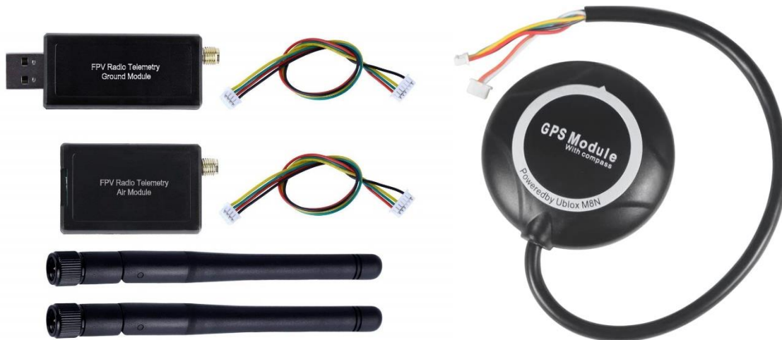
Figure 2.10 433 MHz telemetry module and GPS module.
