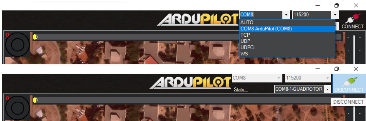
Figure 2.14 Connecting the Pixhawk with Mission Planner.
