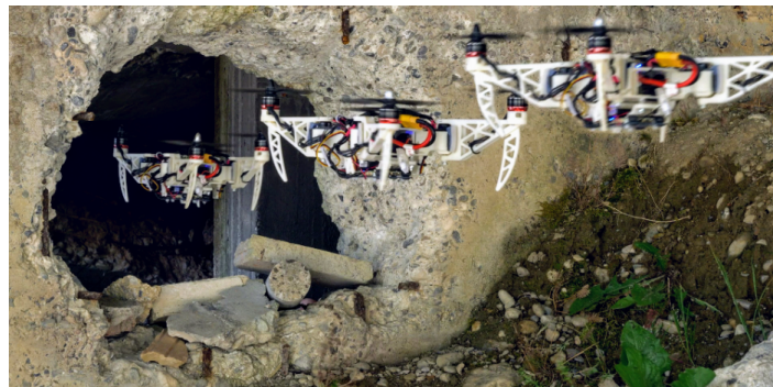
(c) An example of foldable quadrotors that could aid search and rescue in wrecked building.
