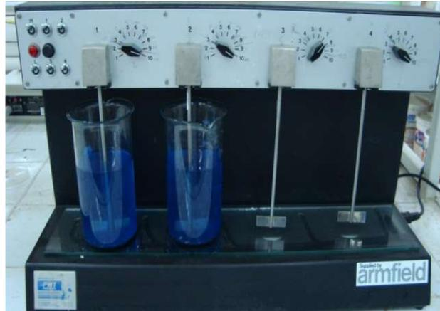
**Figure 4.23:** Aspect de la solution durant la coagulation - floculation
