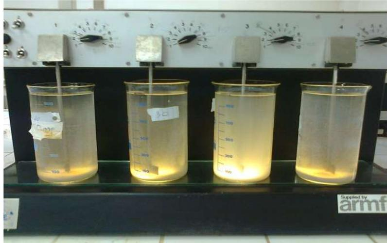
*Figure 3.5: Photo du jar test*
