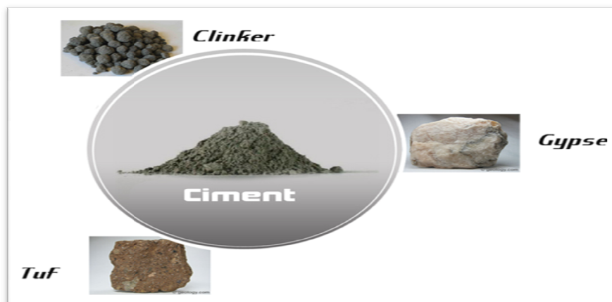
Figure 1.4 :broyage du clinker, gypse et tuf = ciment
