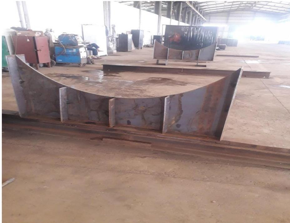
**Figure 3. 5: Fabrication de berceau [Source MAGI]**
