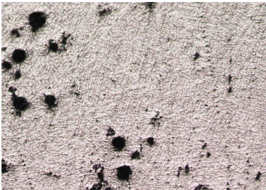
Figure 36 Microstructure de la ZF de T3, X50
