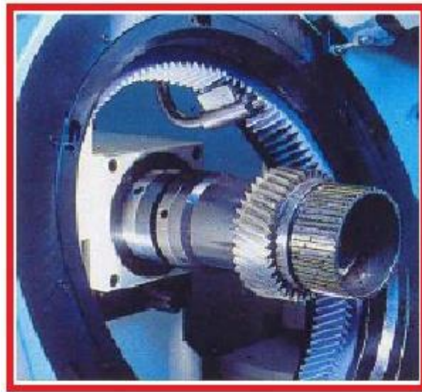
Figure II.22 : Rodage des dentures
