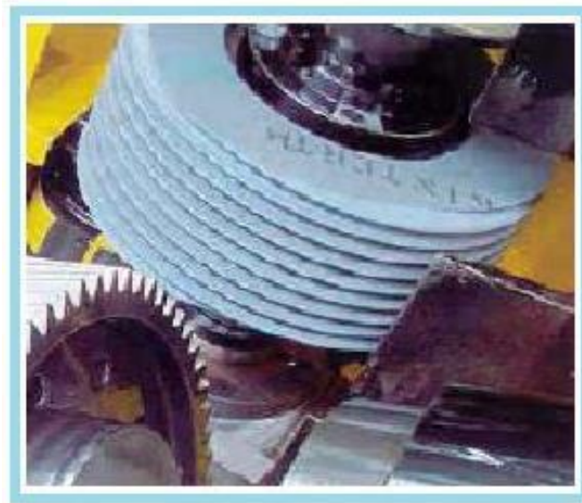
Figure II.21 : Rectification des dentures
