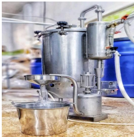
Figure 07 : Alambic d'hydro-distillation (photo originale).
