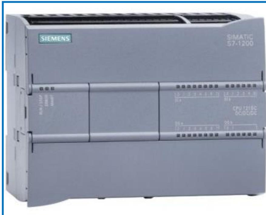
Figure 3.9: API Siemens S7 – 1200COU 1215c .
