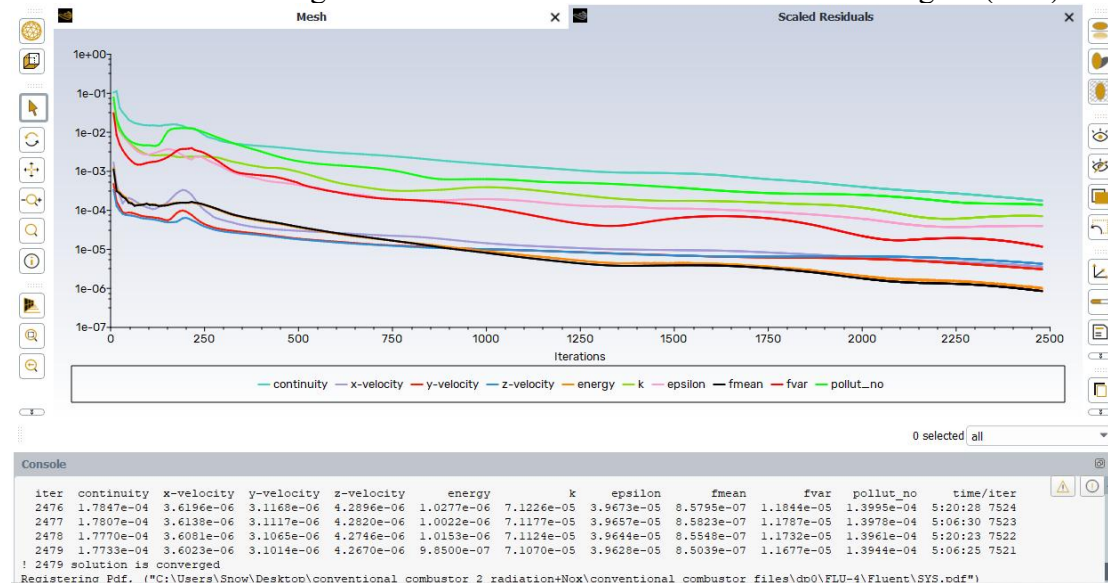
Figure 5.76 residual solution converged for NO x simulation.
