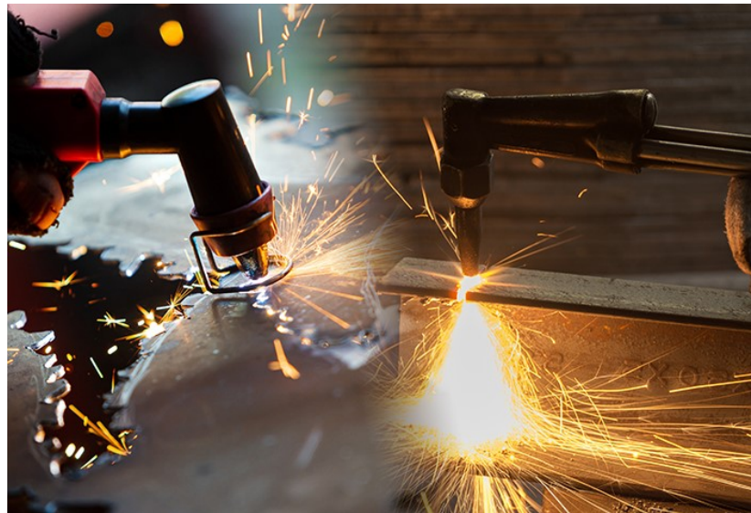
Figure II.4 – Plasma with THC vs Oxy Fuel
