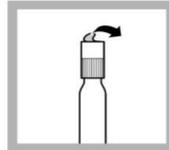
1. Carefully remove the foil from the screwed-on DosiCap Zip.
