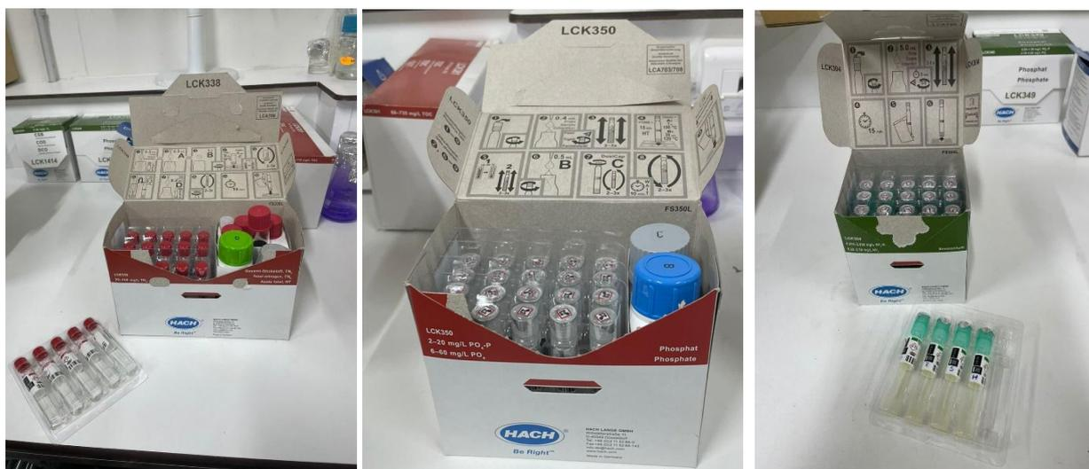
**Figure 2.5** : kits LCK 338 (azote total), LCK 350 (phosphate), LCK 304 (ammonium).
