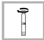
11. Screw a grey DosiCap C on the cuvette.
