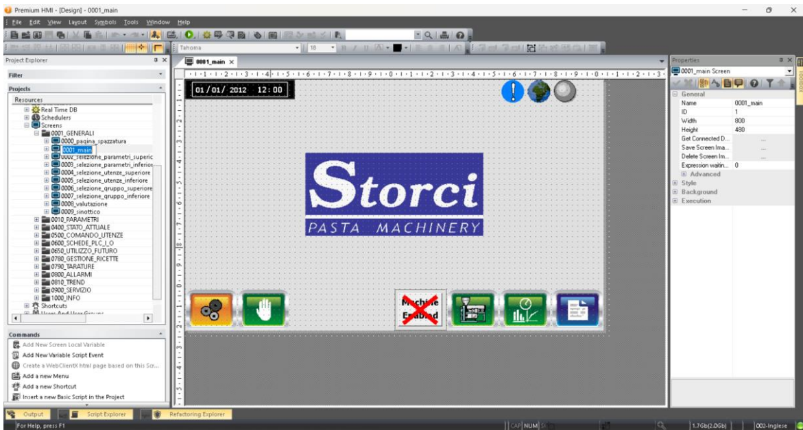
Figure 36: Main Screen (0001_main) in ASEM HMI Interface
