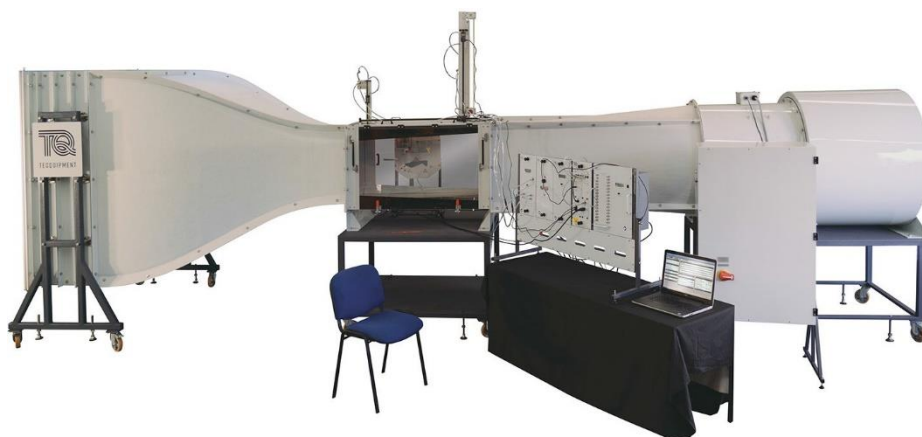
Figure 4. 8The AF1600 with Instruments on the Instrument Frame
