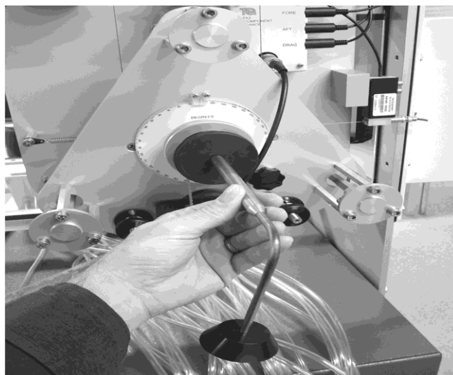
Figure 4. 10 Insert the Model from Outside the Working Section
