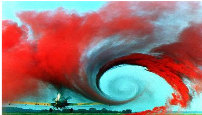
Figure 1. 24 Vortex created by the passage of aircraft wing, which is exposed by the colored smoke (Rafiuddin, 2008)
