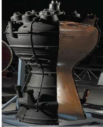
Figure I- 5: Conical nozzle of the V2 rocket.
