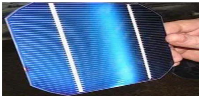
Figure (I.6) : Cellule solaire photovoltaïque monocristalline 156 x 156 mm.
