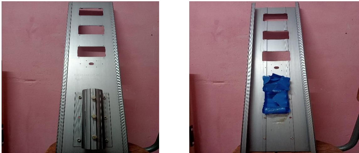
Figure (III.6) : Structure de luminaire solaire All-In-One
