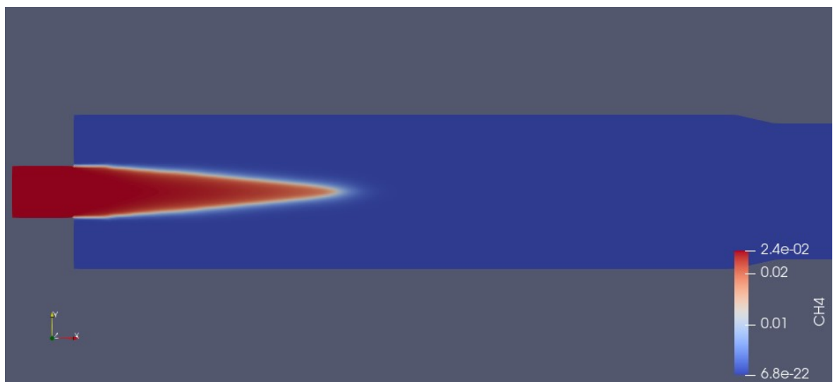
Figure 4. 24 CH4 mass fraction field in reacting flow \Phi = 0.43
