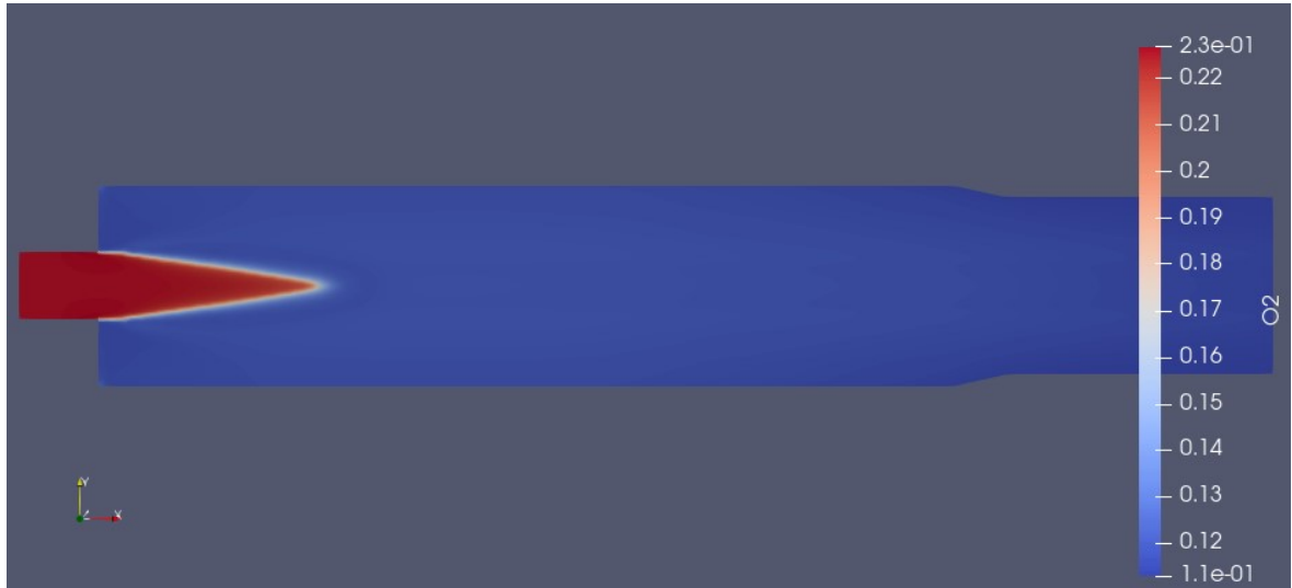
Figure 4. 21 O2 mass fraction field in reacting flow \Phi = 0.56
