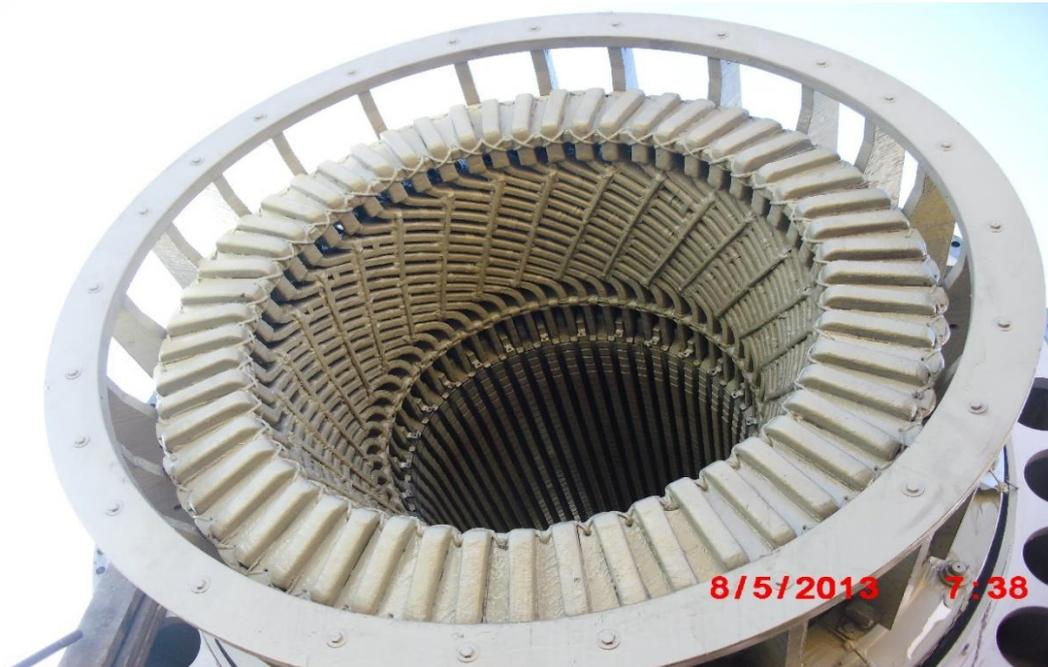
Figure 1.7: Noyau du stator. [6]
