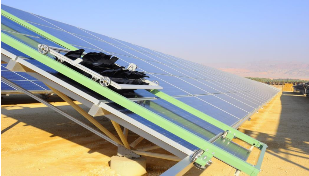
Figure 13: Ecoppia E4 Robot.[36]
