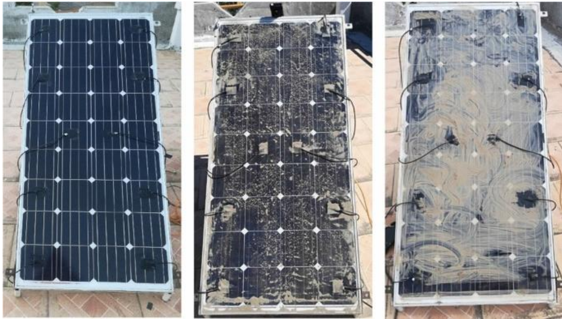
Figure 6: Research about the efficiency loss due to dust and dirt [25].
