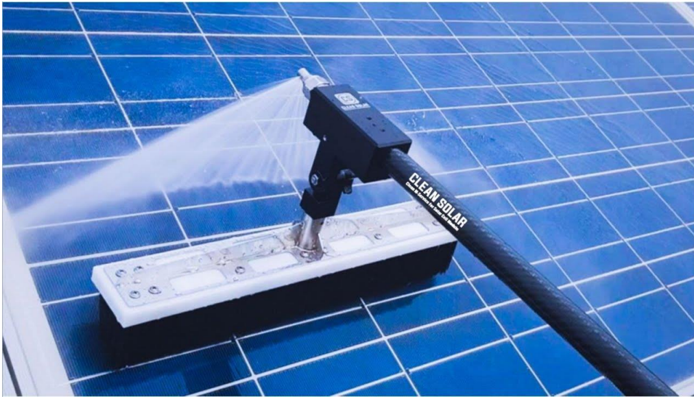
Figure 21: Manual cleaning using Soft-Bristle Brush.[52]
