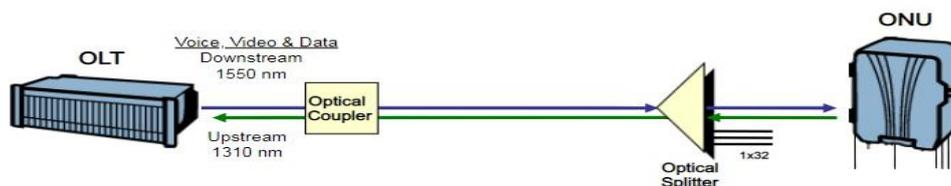
**Figure 2. 15:**architecture du ATM-PON [27]
